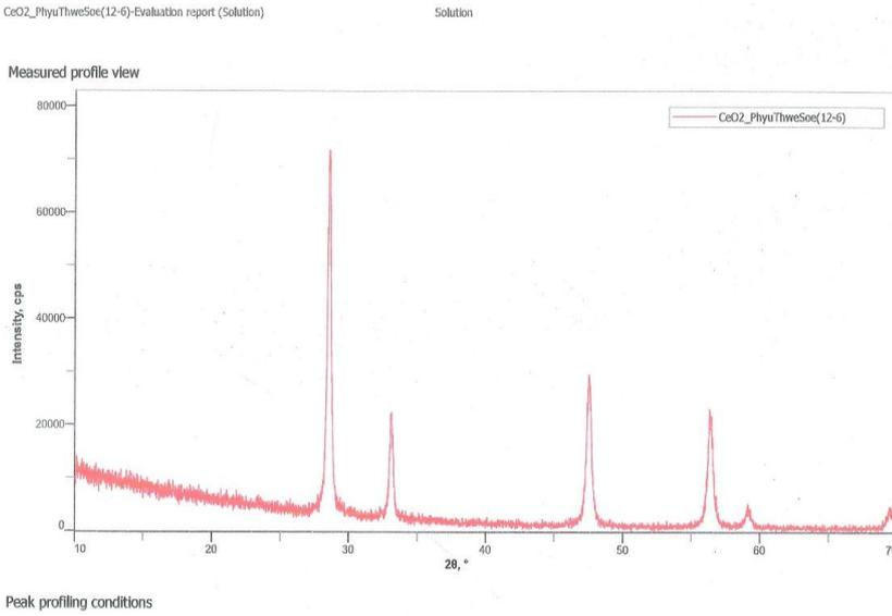
Figure 3. XRD spectrum of Cerium Oxide Nanoparticles
