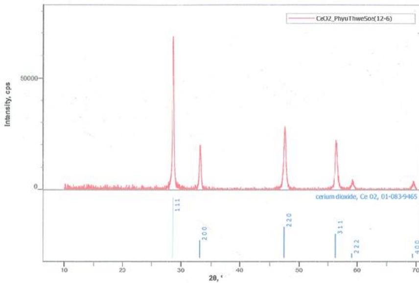
Figure 4. Lattice constants from peaks location and Miller indices of Cerium oxide nanoparticles
