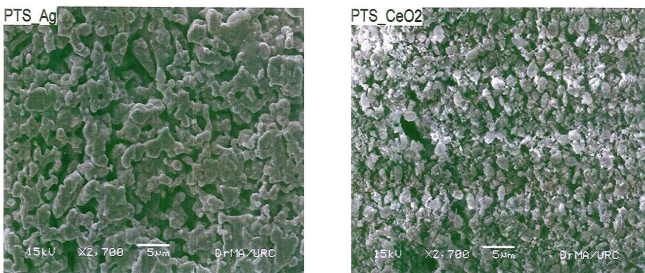
Figure 5. SEM image for Silver and Cerium oxide Nanoparticles
