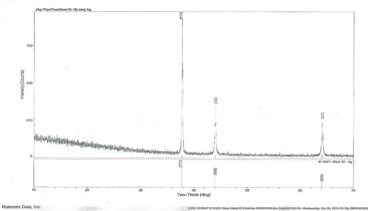
Figure 1. XRD Spectrum of Silver nanoparticles
